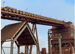
H & B Hungry Boards provide an adjustable barrier to contain rolling bundies travelling on conveyed materials. The height of the hungry boards can be adjusted to suit the gap required to contain the bundies.
