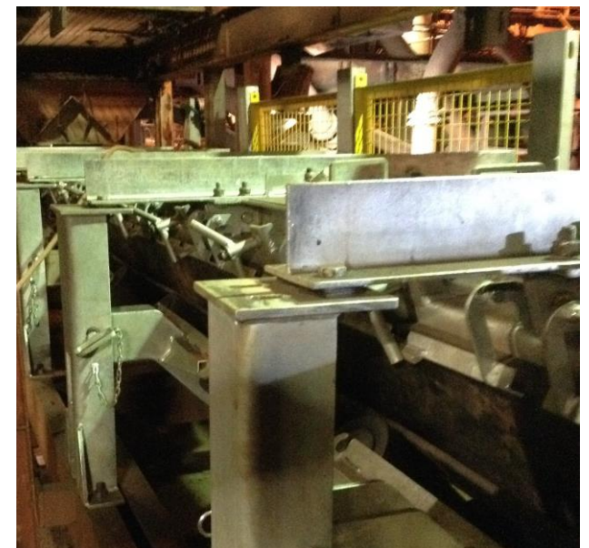
D.D.I. END BRACKETS HOLDING UP SKIRT/DUST COVER SUPPORTS
